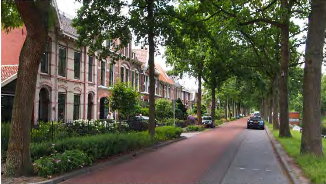
Figure 6-3: Roadway with effective side friction from street trees and shrubs
