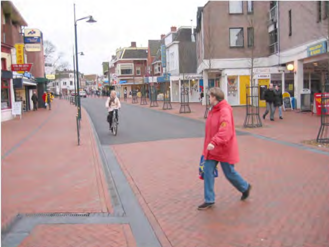
Figure 6-6: Street with change in texture and colour to highlight a transition zone from higher to lower speeds
