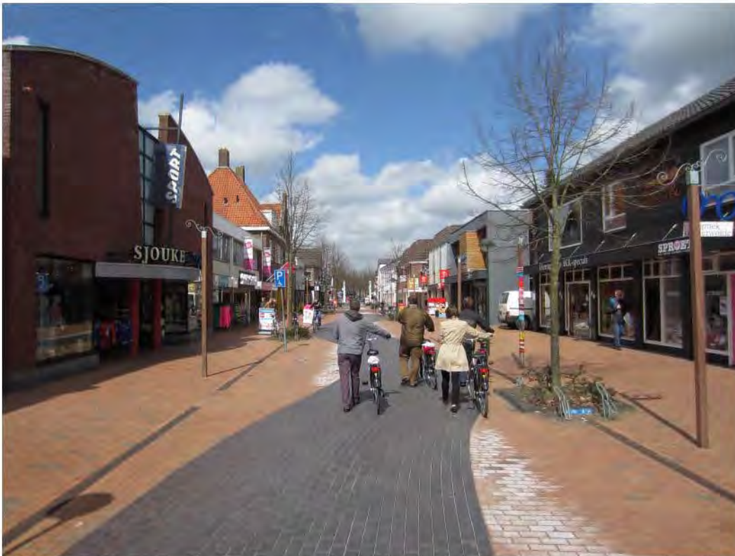
Figure 6-5: Shared Space using trees and planter poles to delineate pedestrian spaces along the edges
